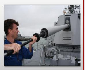
The Ordnance Cleaning System (OCS) can be operated by one serviceman. Its compact design allows for all components to be stored in a weatherproof case that can be stored on a vehicle. The vibrating action of the OCS, quickly removes all residues left behind by firing, leaving the bore in pristine condition. Each kit comes with a set of abrasive, nylon, and stainless steel brushes for both the bore and chamber cleaning of the specified caliber or calibers depending on the user's needs.
