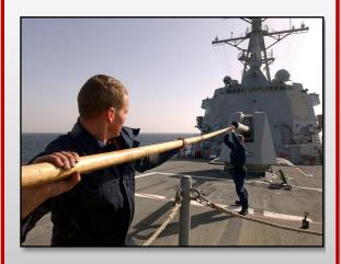
Traditional cleaning practices involve a team of servicemen (2 minimum) using a long rod tipped with a steel brush to "shove" back and forth for many hours to dissolve the rust and gun powder accumulated inside the barrel. This process is time consuming, messy, and arduous, but important preventative maintenance that needs to be completed to keep gun systems in good operating condition, and to keep our servicemen safe.
