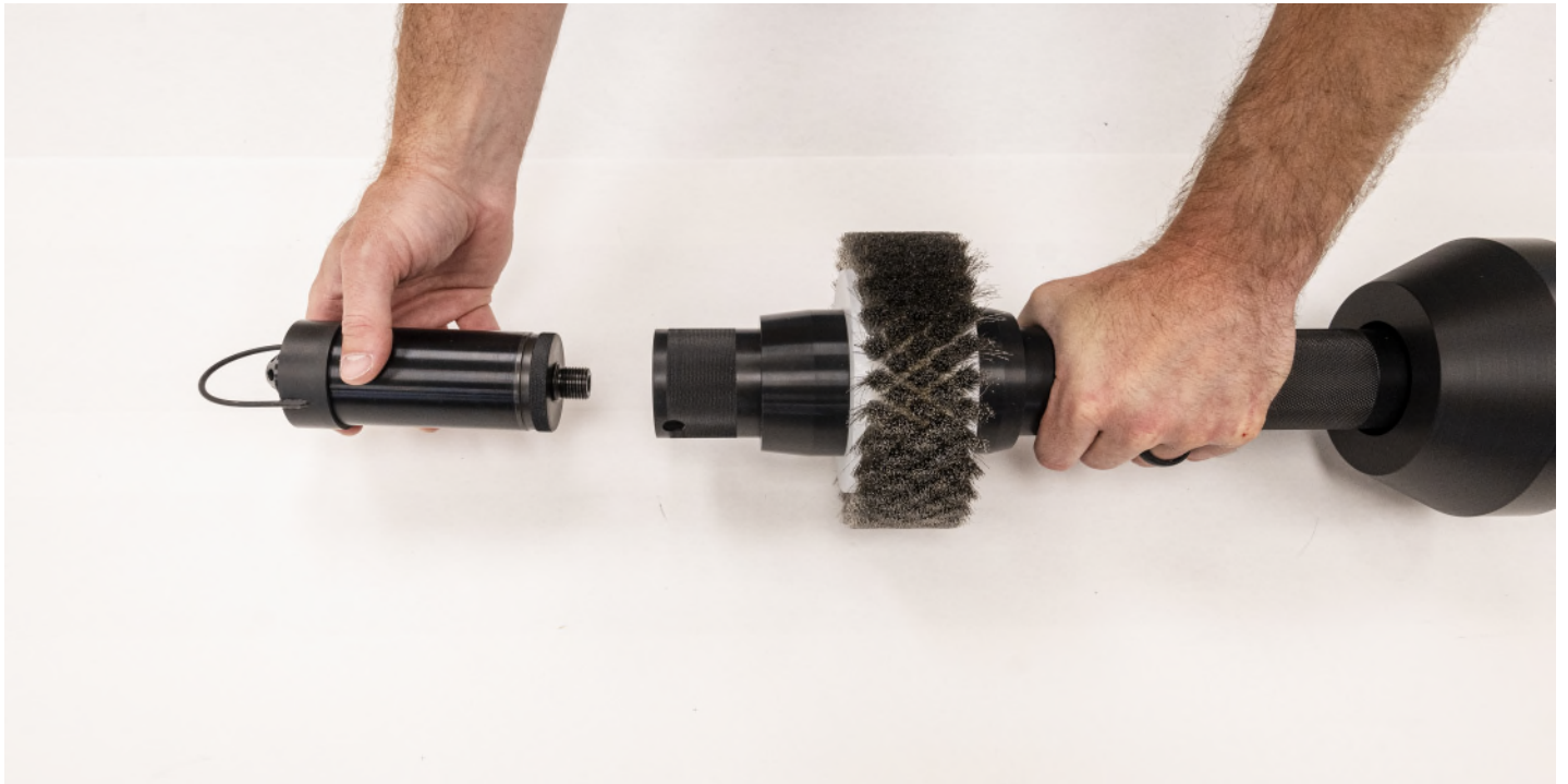
ATTACHING OIL DISPENSER ASSEMBLY TO BRUSH FASTENING SCREW
