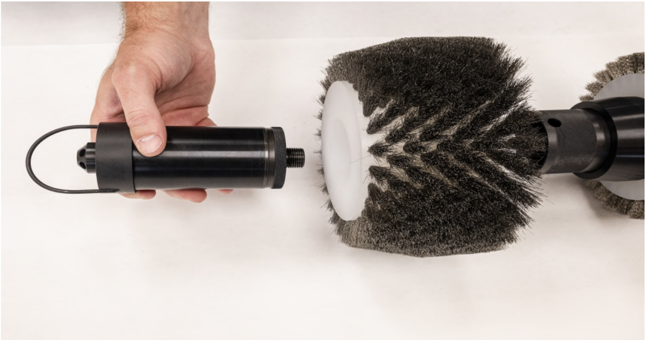
ATTACHING OIL DISPENSER TO CHAMBER BRUSH FASTENING SCREW
